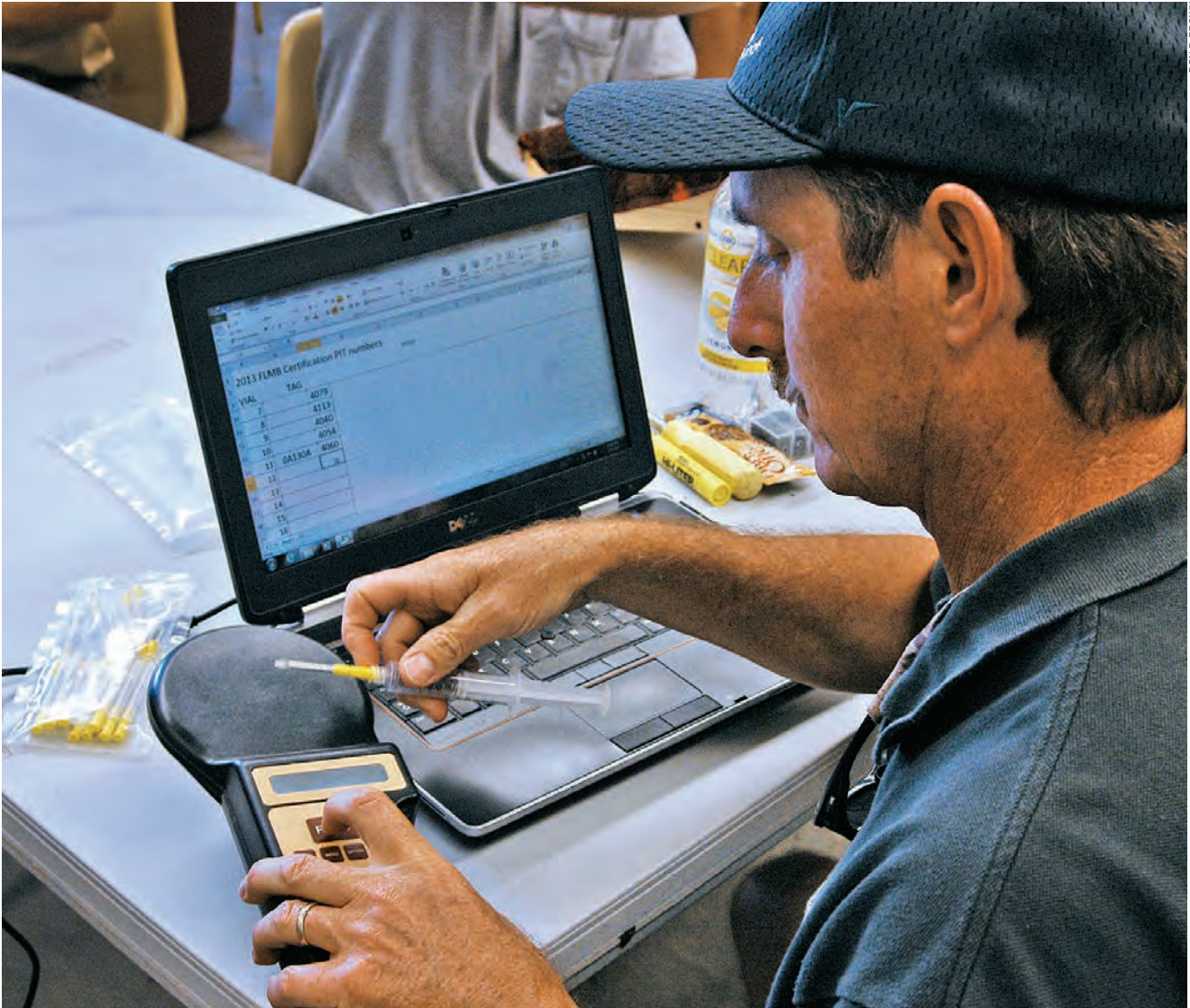
Durant Hatchery manager Gordon Schomer scans a PIT tag inside a syringe and records its ID code in a computer.
