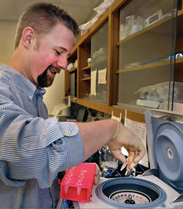
OU research associate Rich Zamor places vials containing fin clip samples into a centrifuge.
