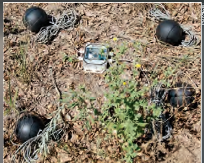
Researchers are using the above device to record operative temperatures across quail habitat. Research similar to this has shown lemon sumac and other shrubs found in mixed shrub communities provide thermal refuge.
