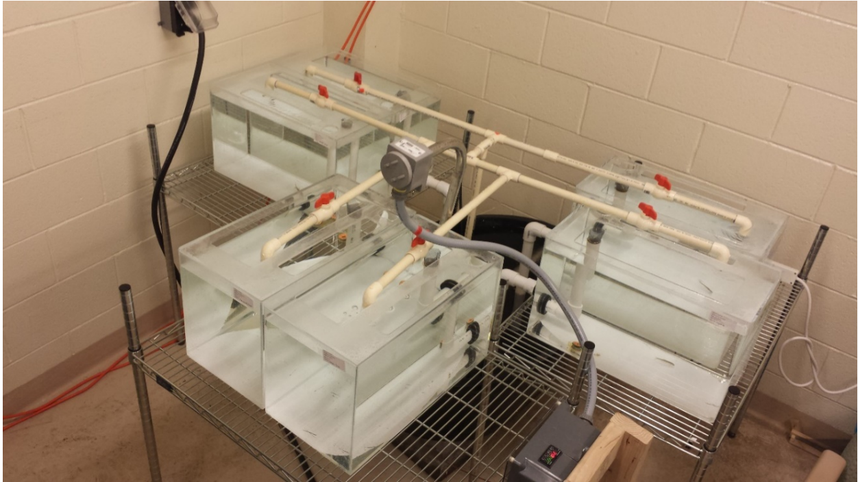
Figure 5. Sump system for testing critical thermal maximum (CTMax) and long-term thermal stress. A pump discharges water into the 37.85-L aquariums and a gravity fed system discharges water into the 189.27-L sump. During CTMax trials, water is heated in the sump by a 5000-W Smartone heater (OEM Heaters, Saint Paul, MN). During long-term thermal stress trials, water is heated in the sump by a 1700-W Smartone heater (OEM Heaters, Saint Paul, MN).
