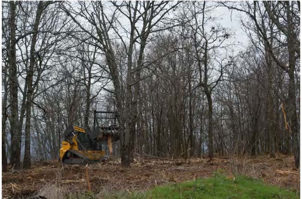
A masticator thins the tree canopy at Cookson Wildlife Management Area. Photo by ODWC.
