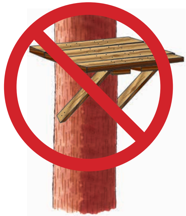
Homemade Permanent Stands in Trees — Should never be used. Wood rots, trees grow and changing weather conditions can cause damage to the stand not seen by visual inspection. Permanent stands and screw-in steps are illegal on wildlife management areas.
