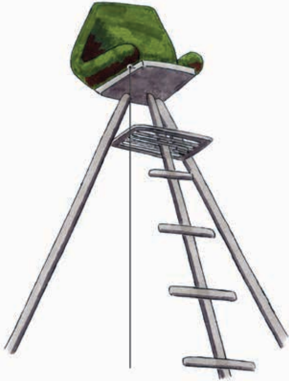
Self-supporting Stands (Tripod Stands) — Used when no trees are available. Needs to be erected on level ground.
